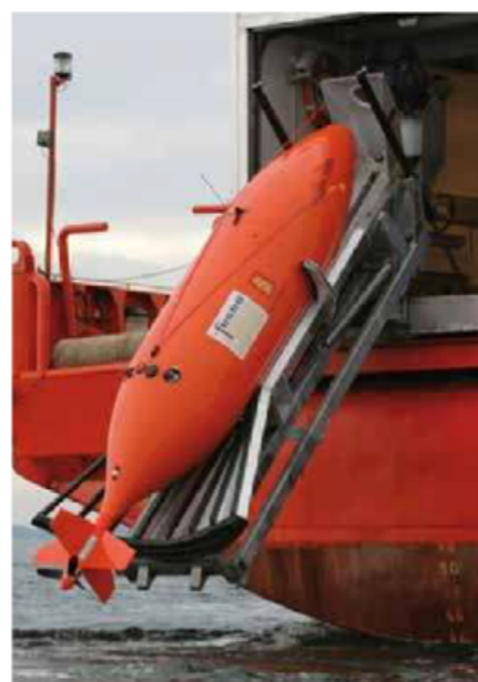
AUV being deployed off back of vessel.
