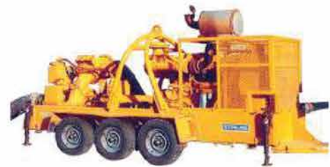
SPP SELF PRIMING DEWATERING PUMPS CAPACITY : 2550m 3 /hr, H=130m
