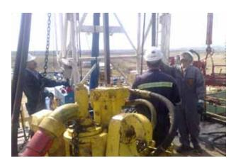
to arrive shortly. Often the gas or oil is holed up inside rock, and the equipment is able to pump fluid and sand at high pressure into the rock to fracture it and create cracks that the sand enters. Once the pressure is released, an environment is created that allows the oil or gas to flow into the well reservoir, significantly increasing the productivity.
