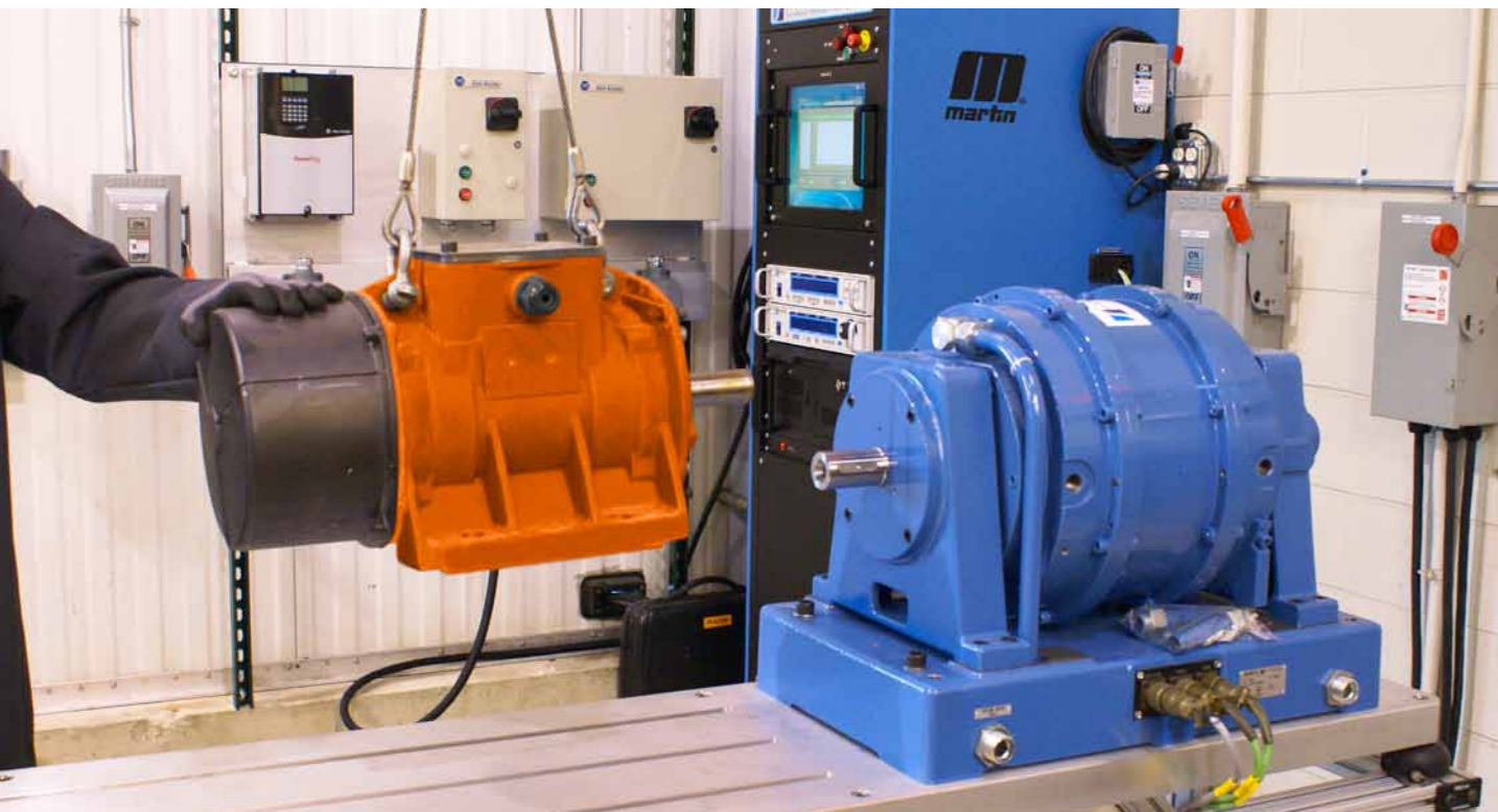
Martin's new capabilities include sophisticated dynamometer testing that allows the company to map the shape and values of an electric motor's torque curve
