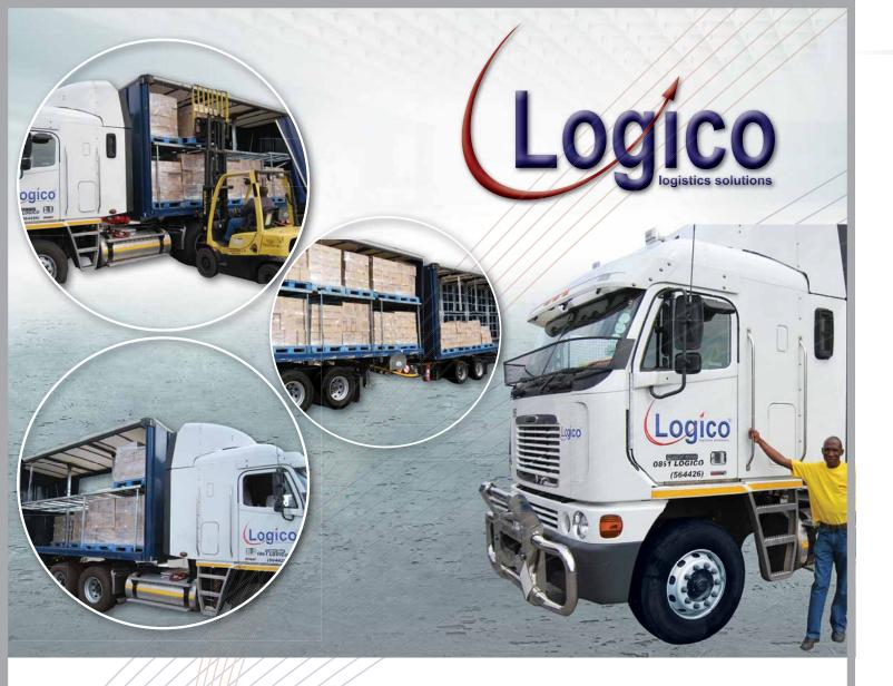
**LOGICO LOGISTICS SOLUTIONS** utilises a patented 72 pallet super link trailer configuration which is designed to allow pallets to be double-stacked, reducing carton damages whilst maximizing vehicle utilisation. The increased utilization significantly reduces carbon emissions as a result of fewer vehicles being required to move the same volume.
