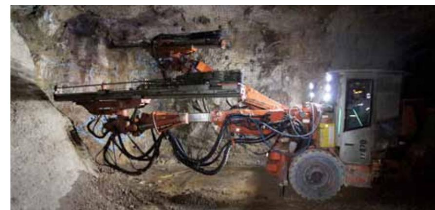
A double jumbo drill is drilling the face for the next shot (explosives)
