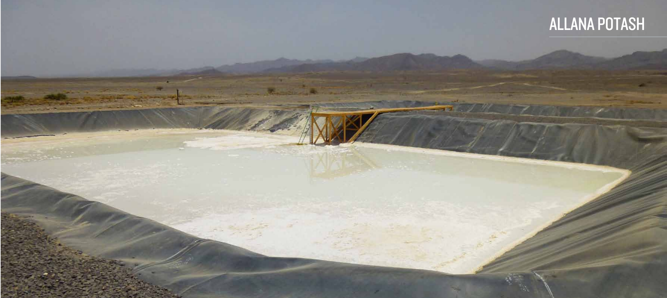
Potash salt and halite crystallization in pilot test evaporation ponds
