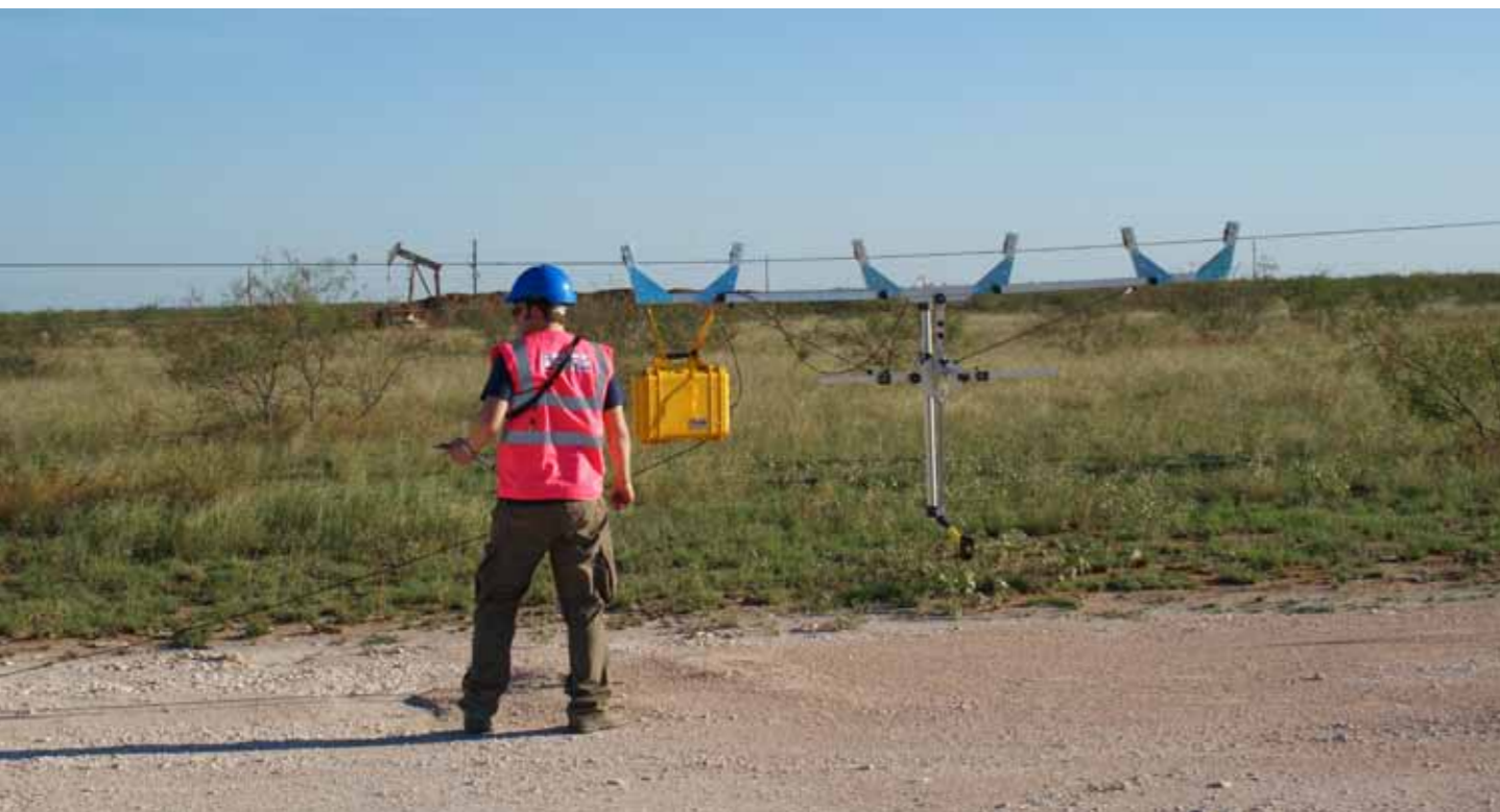
One of Adrok's many onshore surveys in USA. For this survey in Texas, the ADR scanner was deployed from a zipline.
