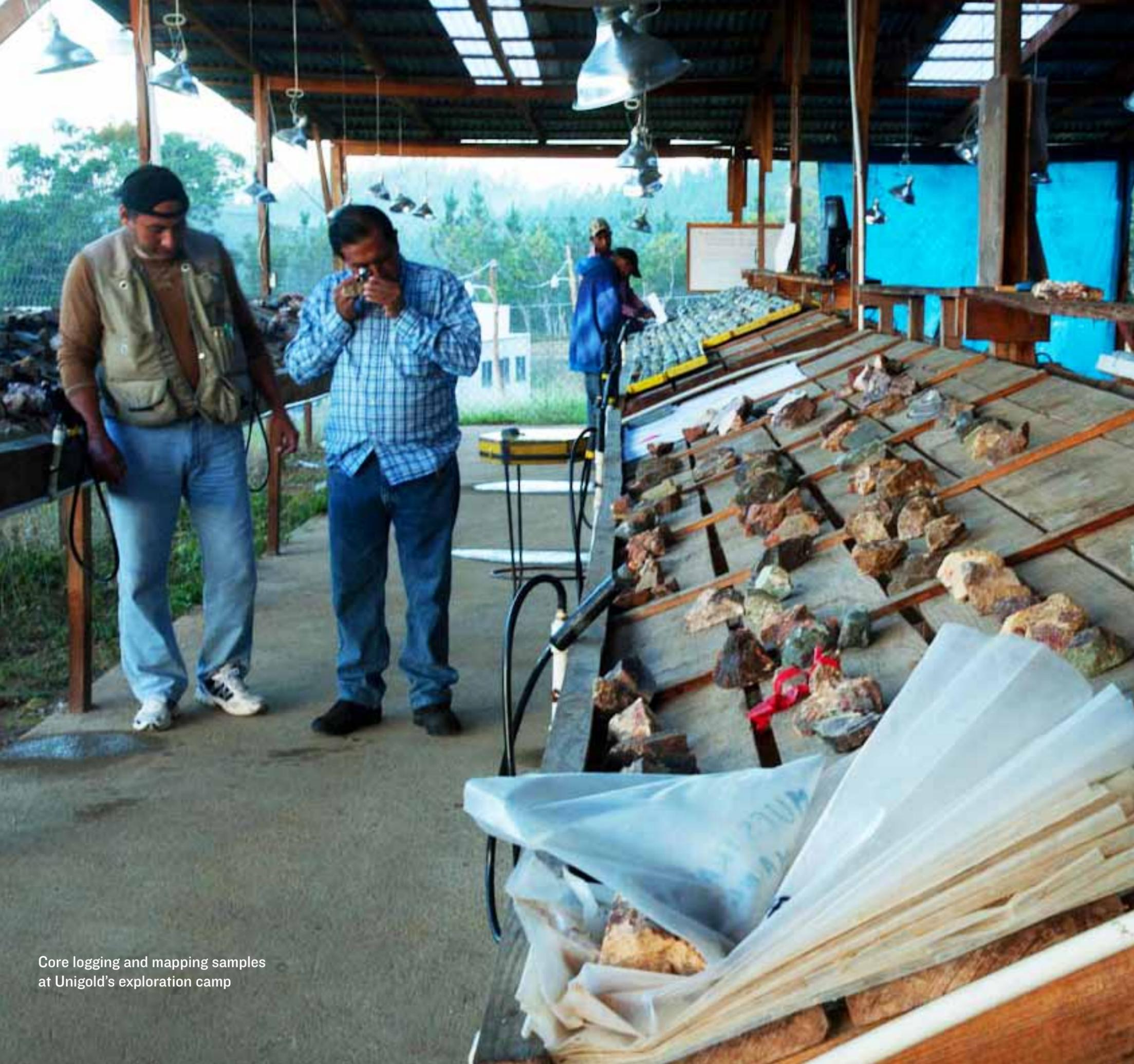
Core logging and mapping samples
