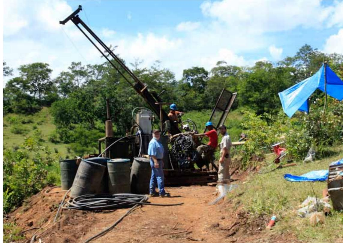
Diamond drill at Lomita Piña, drilling hole LPI7
