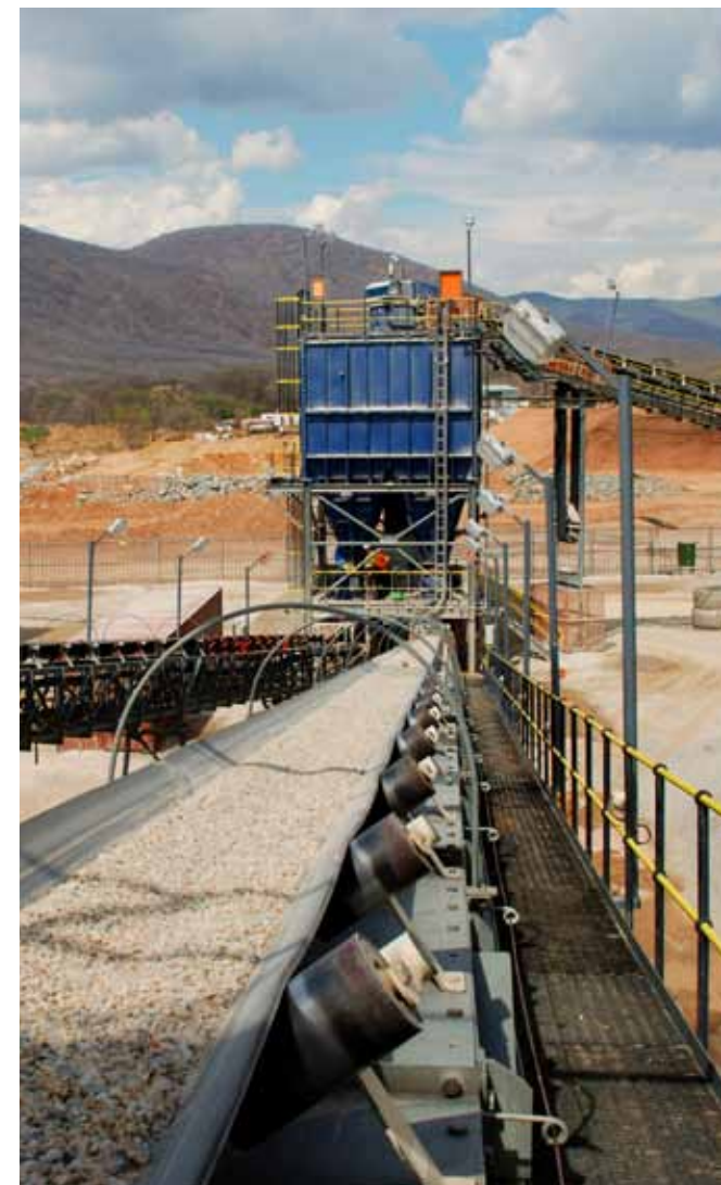
Mill feed bin in production
