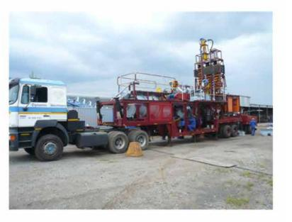
Once on site, our plants require only connections to water and power and can then be switched on immediatly for mineral and ore upgrading and production. (They also have 160KW built in power generators.)
