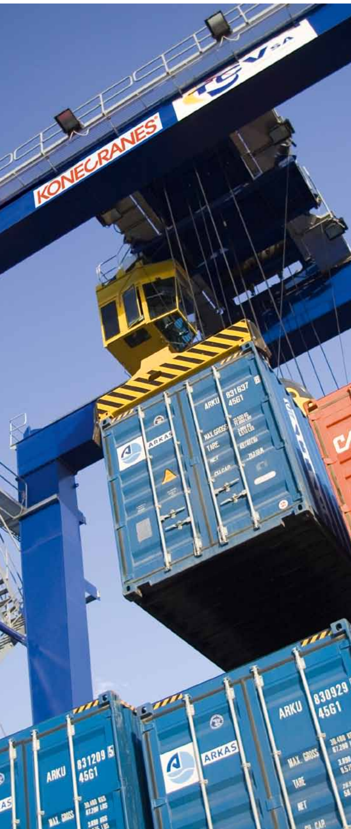
Rubber tyred gantry crane at Valencia, Spain
