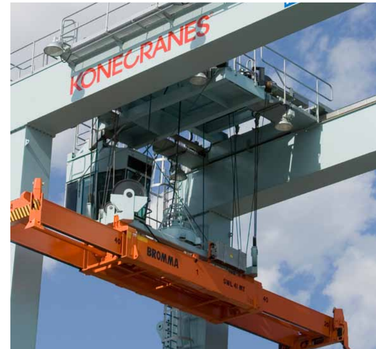
16-wheel rubber tyred gantry crane at MassPort, Boston, US
