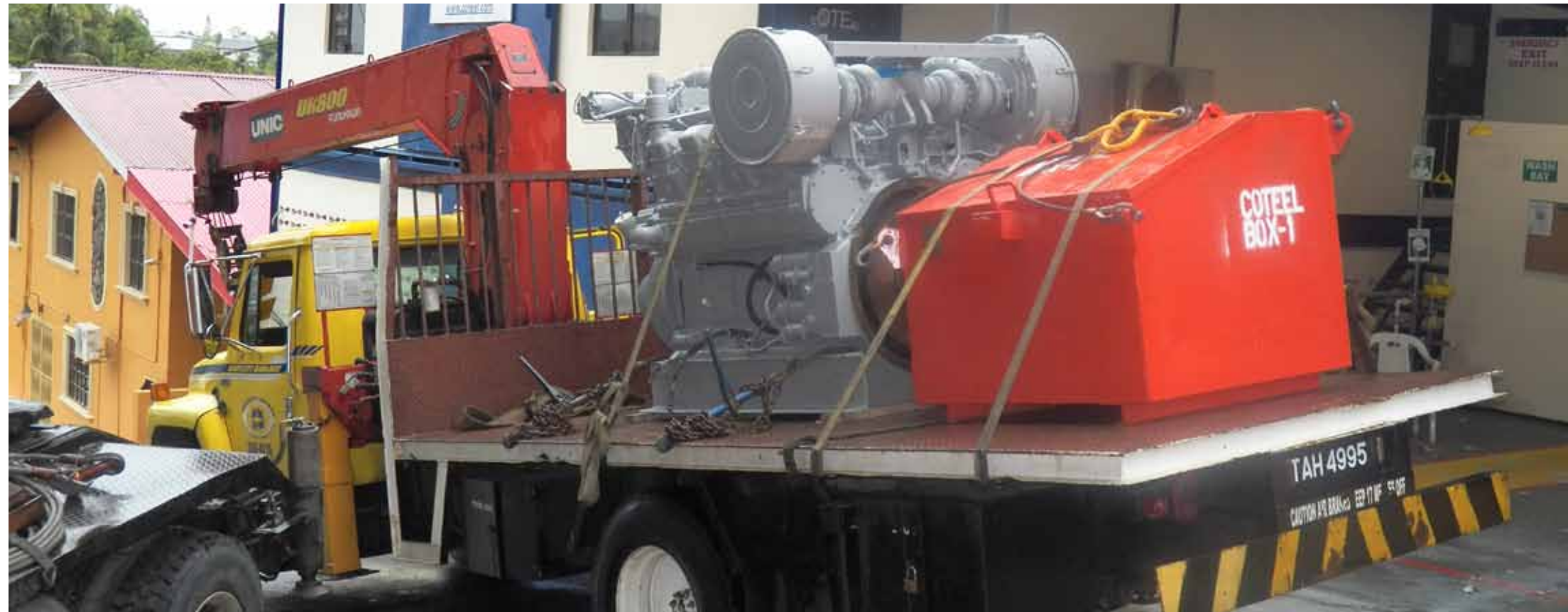
Refurbished CAT 3508 diesel engine transported back to offshore platform for re-commissioning
